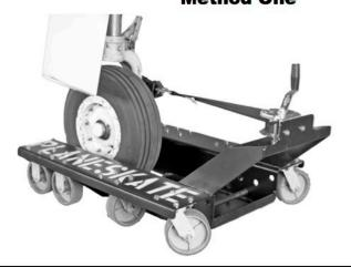
For aircraft 3,500lbs. / 1,580kg or less, wrap the axle strap around the gear leg then attach the winch strap to the axle strap and carefully tighten.
