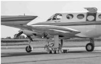
Wheel the 4K PlaneSkate<sup>™</sup> up to the distressed tire, chock both forward wheels of the PlaneSkate<sup>™</sup>, and tow the distressed aircraft onto the 4K PlaneSkate<sup>™</sup> tray. Once in place, secure aircraft with winch strap and any additional straps as necessary
